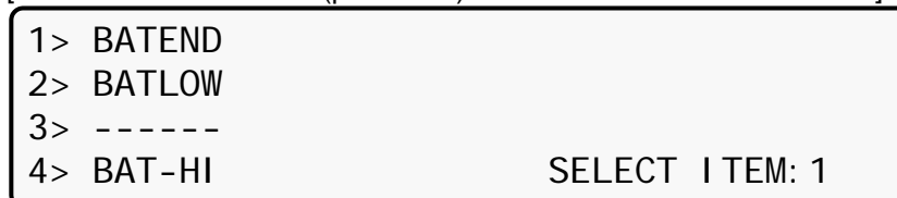
Figure 141: Battery floating charge alarm setup menu
