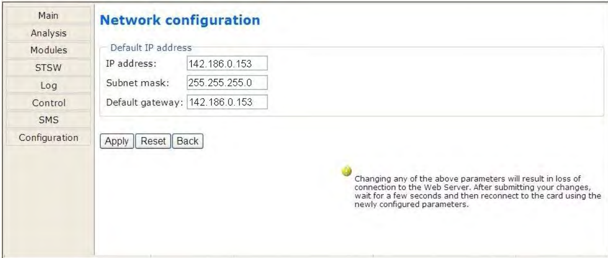
Figure 312: Configuring network communication parameters
