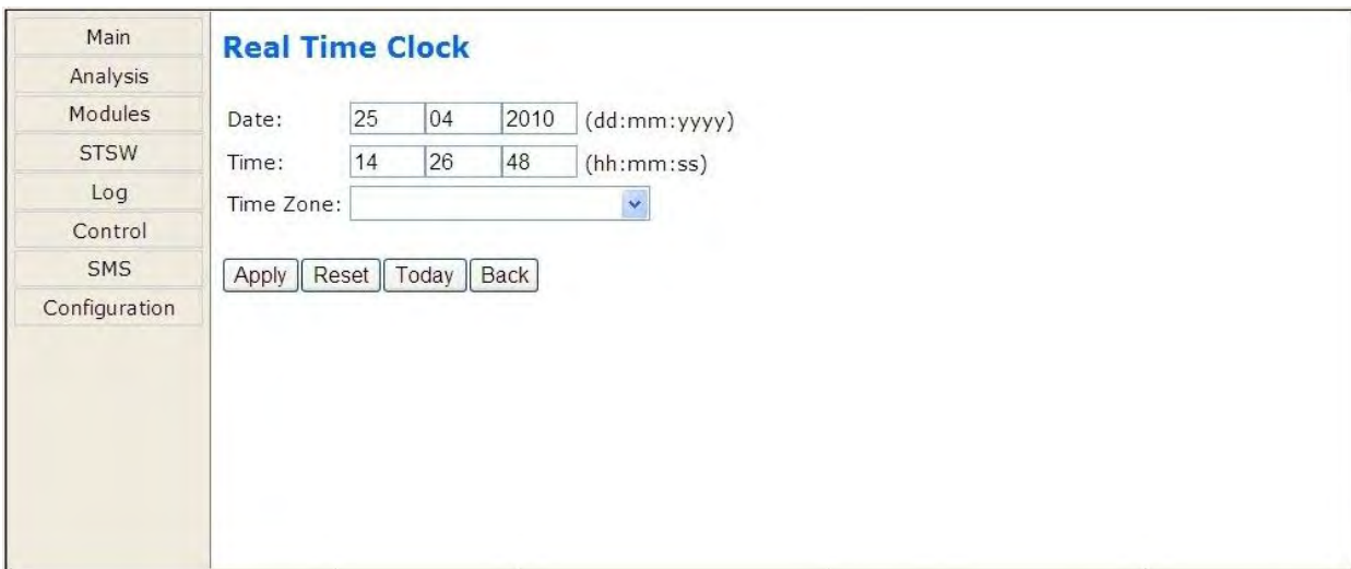
Figure 313: Setting the Power+ internal date and time
